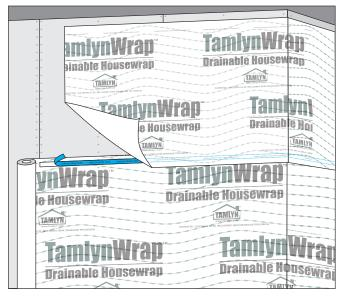
With this in-place unroll the next course of TamlynWrap<sup>™</sup> maintaining the required 6" of overlap, with fastening stopping 9" from the bottom of this course allowing for it to be folded up.
