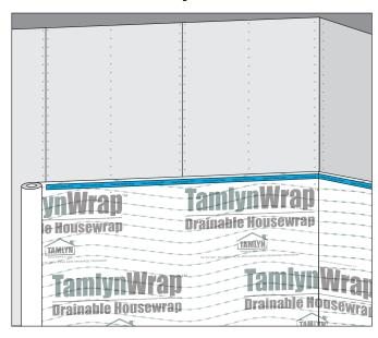
Unroll first course of TamlynWrap™ with spacers facing the exterior and fasten to sheathing with cap-fasteners. XtremeSeam Tape™ is applied to the first course by removing one side of the release paper and for best results lay down with a foam roller or hand applicator.
