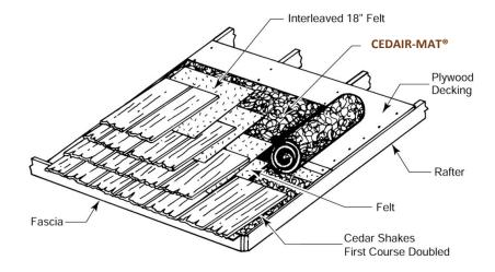
Note: Recommended on a 4/12 roof slope or greater.
