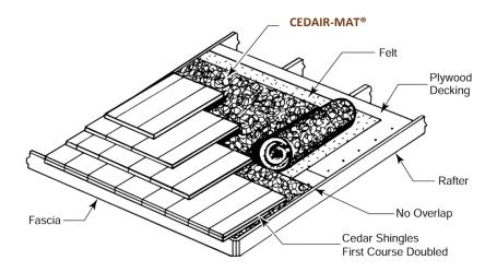
Note: Recommended on a 3/12 roof slope or greater. Shingle installation can be used with 3-ply tapersawn shake application.
