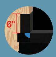
• To use HydorCorners instead of patches, place a HydroCorner in each sill corner and fasten in place with a staple. Install HydroFlash UV+ 9" to extend at least 6 inches up the inside of each jamb inside the window opening.
